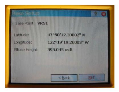
This is your "<u>Base Station</u>" reference position (in Lat. and Long.) to be stored in your job. Click **"Set"** to accept the remote "Base Station" position to continue on with the VRS survey.
