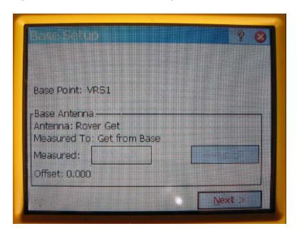
The next screen is the "<u>Base Station</u>" antenna type and measure up. You can not change this since the server sets this automatically. Click "**Next >**" to bring you to the "<u>Base Station</u>" coordinates (in Lat. and Long.) that the server set for you.
